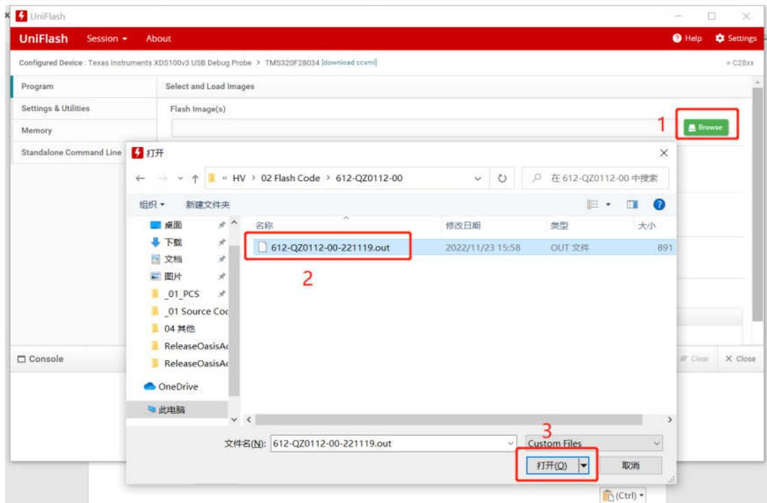
5.click the “load image” button to start the download procedure, when the download procedures are successful, it will show the download result as below.
